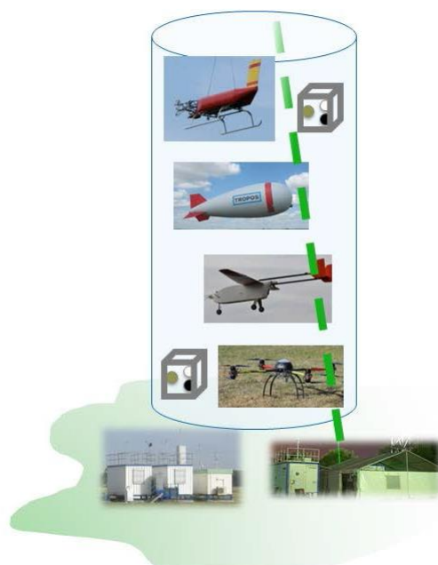
Figure 5: Schematic of the Melpitz column: Combination of ground-based in-situ, ground-based remote sensing and airborne measurements of aerosol particles and their optical properties.
