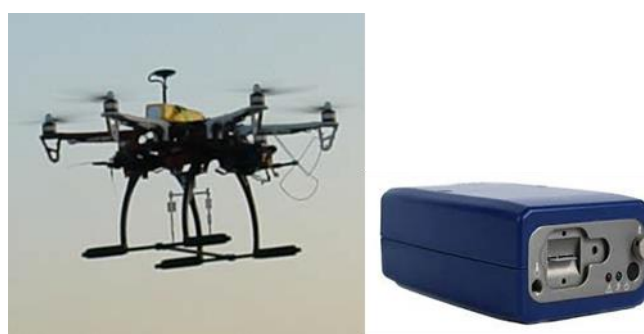
Figure 13. NOA UAV (left) and Miniature black carbon aethalometer (ETS AE51) (right), at the ACTRIS-2 JRA1 Athens smog campaign.
