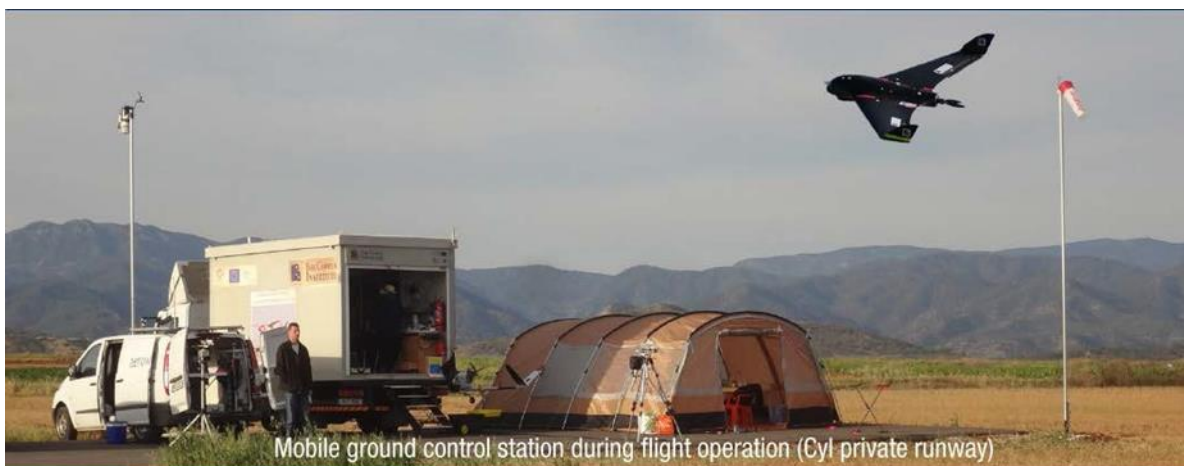
Figure 20: UAV flight operation in Cyprus with the Cyl mobile ground control station (April 2016). The black UAV is a fixed wing foam Skywalker X8.
