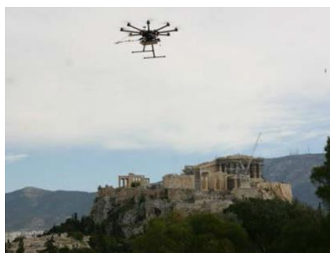
Figure 11. Picture of the Cyl rotary wing UAV equipped with Absorption sensors, T/RH/P probes and video. Photo taken from Thissio.
