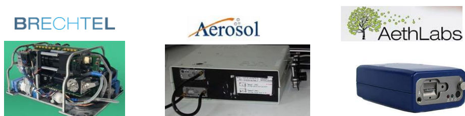
Figure 12. Pictures of the 3 miniaturized absorption instruments tested onboard the Cyl UAV. From left to right: STAP (from Brechtel), DWP (dual-wavelength prototype by Aerosol doo), and AE51 (by Aethlabs).
