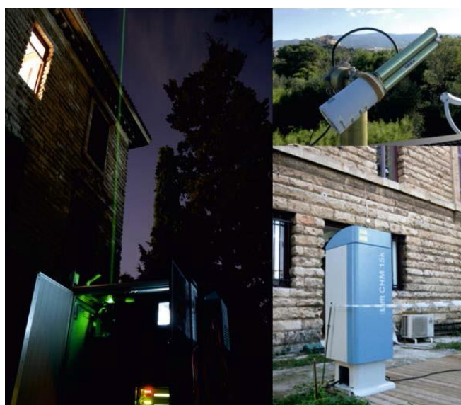
Figure 15. PollyXT NOA lidar (left) at the Thissio site, CIMEL sunphotometer (upper-right) and Lufft Ceilometer (lower-right) during the ACTRIS-2 Athens smog campaign.
