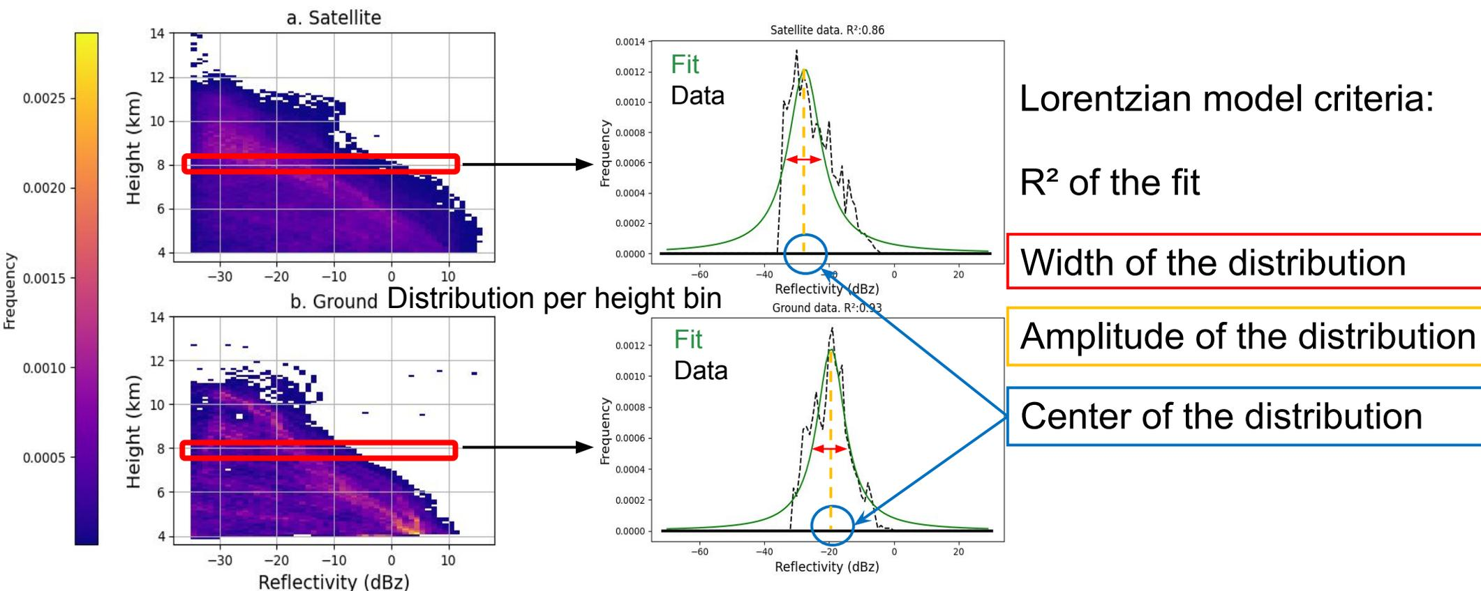
**Fit with a Lorentzian model** to sort data (threshold based):
