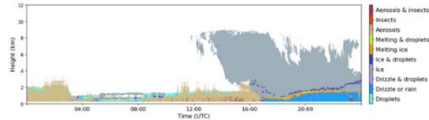
Radar and lidar detection status
