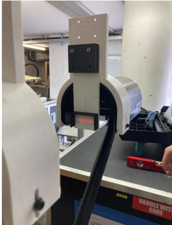
Dropping device also provides a tool to make sure that laser band is well aligned.
